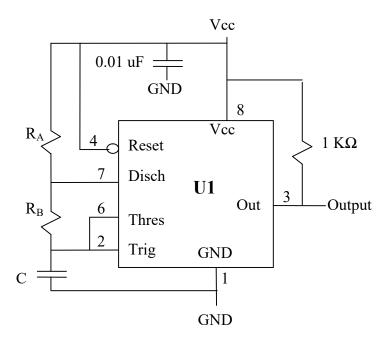
Calculate and draw the clock signal based on the formulas provided. Compare the clock signal waveform observed on the output pin of NE 555 with the calculated waveform. Explain reasons for differences between the two waveforms.
