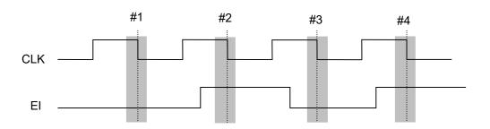
3U. Draw a clock signal CLK with five 0-to-1 timing events, a nonzero setup time,  $t_{su}$ , and a nonzero hold time,  $t_{h}$ . Also draw one excitation input signal EI that follows the sequence 10110 and meets the setup and hold time requirements. In the excitation input, the first bit in the sequence (1) occurs in time for the first clock timing event, the second bit in the sequence (0) occurs in time for the second clock timing event, and so forth.
