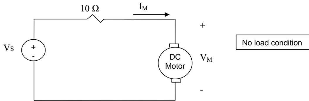
Starting  $V_s$  at 0 volts, increase  $V_s$  and measure  $I_M$  and  $V_M$  until the DC motor is rotating continuously. Reverse the process and measure the value of  $I_M$  and  $V_M$  as you decrease  $V_s$  until  $V_s$  reaches 0. Note the status of DC motor as you are changing  $V_s$ .
