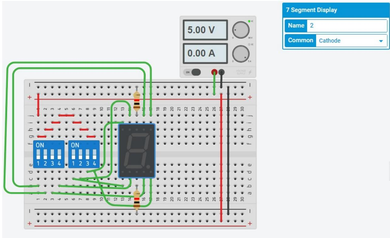
b) Implement the following circuit in TinkerCAD using CD4511 (BCD to 7-segment display driver - common cathode). Simulate the circuit and generate a table that matches all binary equivalents of switch values (1 Msb ... 4 Lsb) with observed numbers on the 7-segment display.
