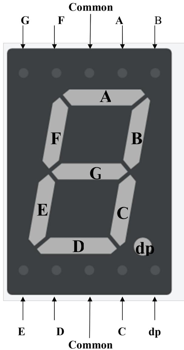
*Notes: If you plan to use CD 4511 display driver, you need to set the 7-segment display to “Common Cathode”. In this mode commons are grounded and high voltage at inputs A-G will turn on the corresponding segment.*
