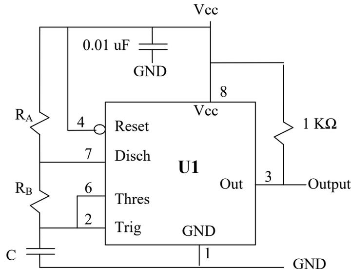
Calculate and draw the clock signal based on the formulas provided. Compare the clock signal waveform observed on the output pin of NE 555 with the calculated waveform. Explain any differences between the two waveforms.
