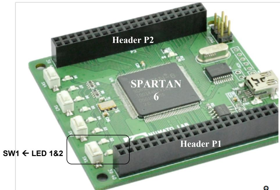
The Board has a 100 MHz built-in clock that is connect to SPARTAN at pin 126. So by adding the following statement to your design's .ucf file, you get access to CLK period of  $10^{-8}$  seconds (50% duty cycle).
