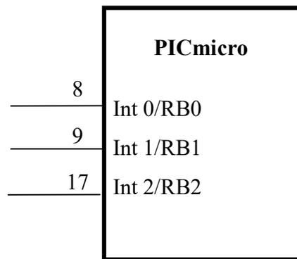
The high priority interrupt vector is at 000008h program memory location and the low priority interrupt vector is at 000018h program memory location. Interrupt vector is the location that PC will be set to after an interrupt has occurred and has been acknowledged.
